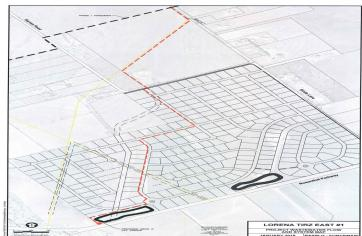
Description of Project: Loera Home Builders will develop a site of 220 acres adjoining the initial TIRZ #1 Phase I project site. Thus the TIRZ #1 was expanded and a Phase II Sanitary Sewer project was initiated. The Phase II Expanded Basin G Sanitary Sewer is 7,450 feet in length (1.4 miles). Loera Home Builders, the City of Lorena, and McLennan County participate in the project financing. This TIRZ project is expected to attract 270 luxury homes at a value more than \$500,000.
